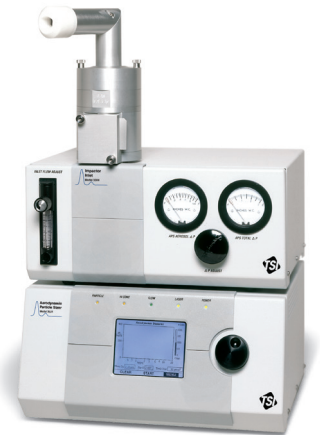
APS spectrometer with optional impactor inlet (Model 3306) for MDI/DPI aerosol analysis.
