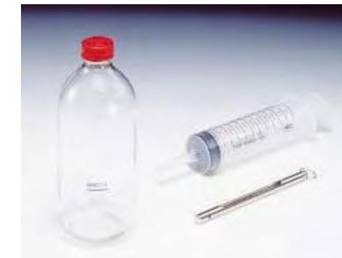
P-20 includes : Resinous gas collector, one collecting bottle and thermometer
