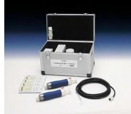
During a disaster, the rescue team may be at risk from invisible toxic gases. The "Harmful Gas Detector for Disaster Relief" can measure toxic gas levels easily and quickly at the disaster scene.
