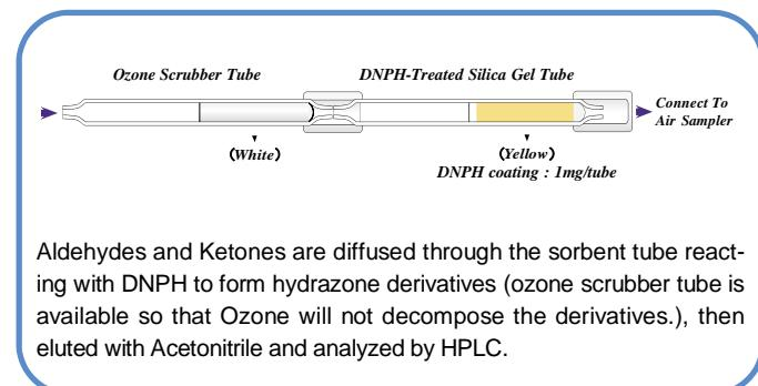
Aldehydes and Ketones are diffused through the sorbent tube reacting with DNPH to form hydrazone derivatives (ozone scrubber tube is available so that Ozone will not decompose the derivatives.), then eluted with Acetonitrile and analyzed by HPLC.
